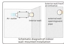
2.The ceiling/wall mounting of the fresh air fan is installed outdoors, the wall is drilled, and the air inlet of the ventilation pipe is connected to the indoor.
